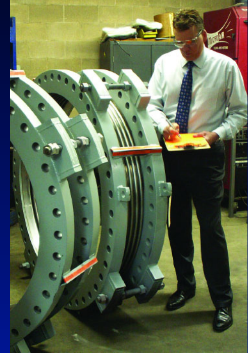
Custom Designed Joint: 30" nominal ID x 36" Fx F, expansion joint with stainless steel liner. Custom elliptical steel flanges, 35" x 50 Fx F" with control rods. Design 150 psi @ 650°F
