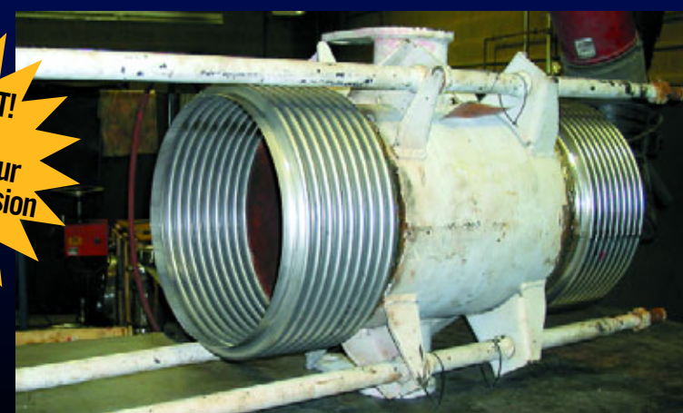
20" Universal tied expansion joint being rebuilt with radiograph bellows.
