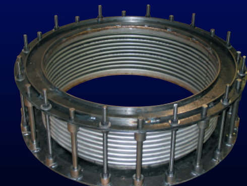
Custom Designed Joint: 30"x14", 316 stainless steel bellows with custom 3 1/2" O.D. carbon steel flanges with groove for carbon sealing ring. Design 1 psi @ 200°F for 2 1/2" of axial compression.
