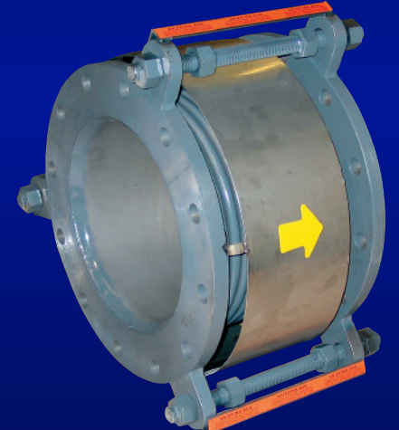
Custom Designed Joint: 16"x13 1/4" Fx F, 321 stainless steel bellows and flow liner, 150# flanges with control rods and exterior shroud. Design 150 psi @ 600°F for 2" axial compression.
