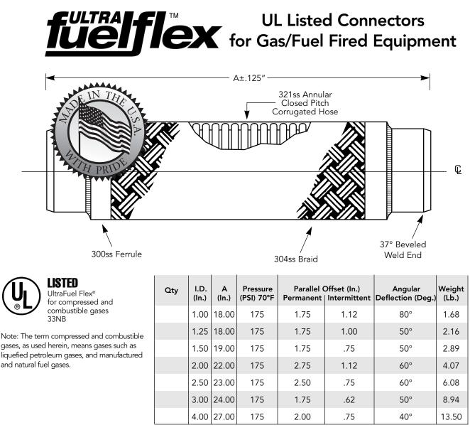
\*Working pressures shown for the hose and braid are based on an operating temperature of 70°F (21°C) with a 5:1 safety factor.
