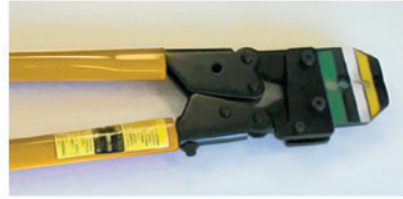
Color coded, factory cable cutter & crimper to meet cable specifications
