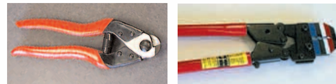
Color coded, factory cable cutter & crimper to meet cable specifications
