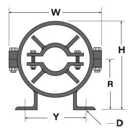
NOTE: The recommendations given for pipe anchors and guides represent the minimum requirements for controlling pipelines which contain expansion joints and are intended to protect the expansion joint and pipe system from abuse and failure. However, additional pipe supports are often required between the pipe guides in accordance with accepted piping practices.
